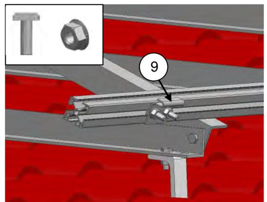
For fixation of each further collector a **lower fastening sheet** is mounted at the appropriate distance 771 mm (1154 mm to the centre of the next collector) to the horizontal rail.
